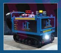
This emergency stop safety feature ensures that at NO time will the operator of this unit be exposed to uncontrolled hydraulic energy as the remote is the only point at which the power can be reactivated.
